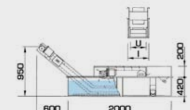
NV7 - NV8 - NV9 Nastro vasca particolari galleggianti e non galleggianti Conveyor with cooling tank for floating and no floating parts
