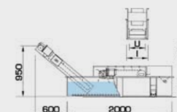
NV4 - NV5 - NV6 Nastro vasca particolari galleggianti Conveyor with cooling tank for floating parts
